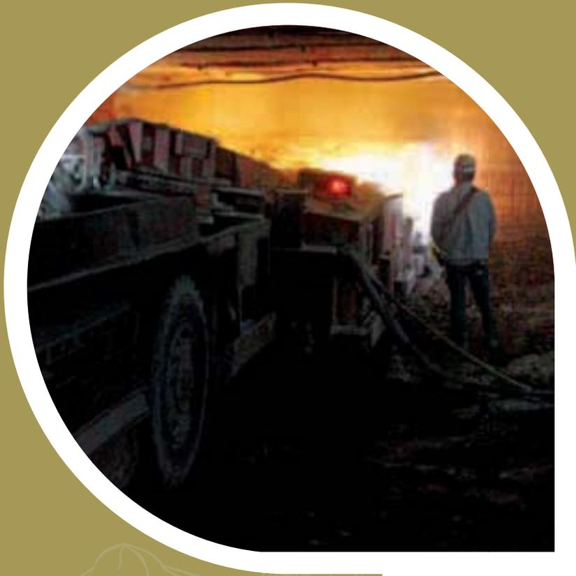
**A** continuous miner, less productive but more flexible than a bore miner, fetches the trona and deposits it in a shuttle car, from where it is transferred to a conveyor belt. The Green River facility sits on the 'mile-high' prairies of southwestern Wyoming, home to the largest reserves of trona ore in the world — 60 billion tonnes spread over 1,000 square miles, at depths of up to 1,800 feet.
