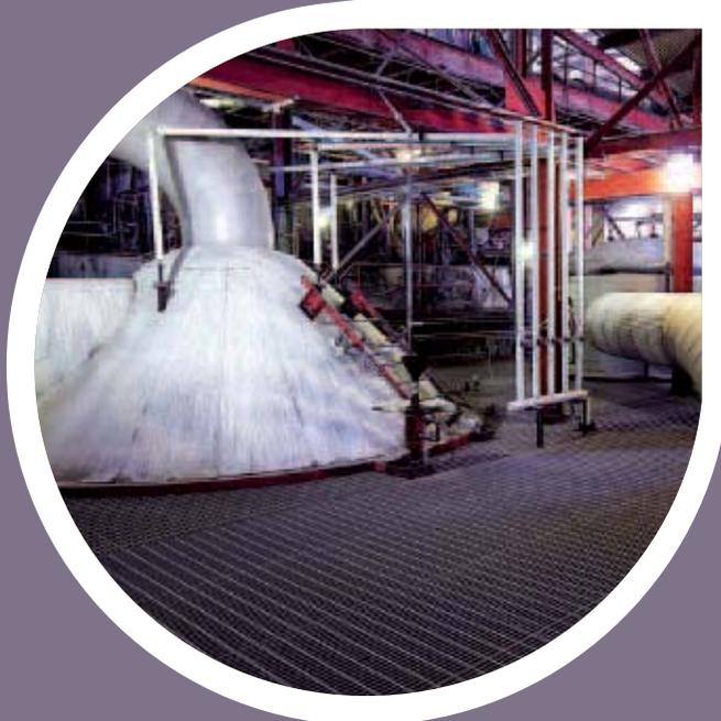
**W**ith shale and other contaminants removed from the liquid substance obtained in the purification process, the water used to dissolve the ore can now be removed. Evaporators, such as those seen here, boil the solution, leaving behind soda ash crystals. These crystals show up as a kind of slurry. Any remaining water is separated from the crystals in a centrifuge.
