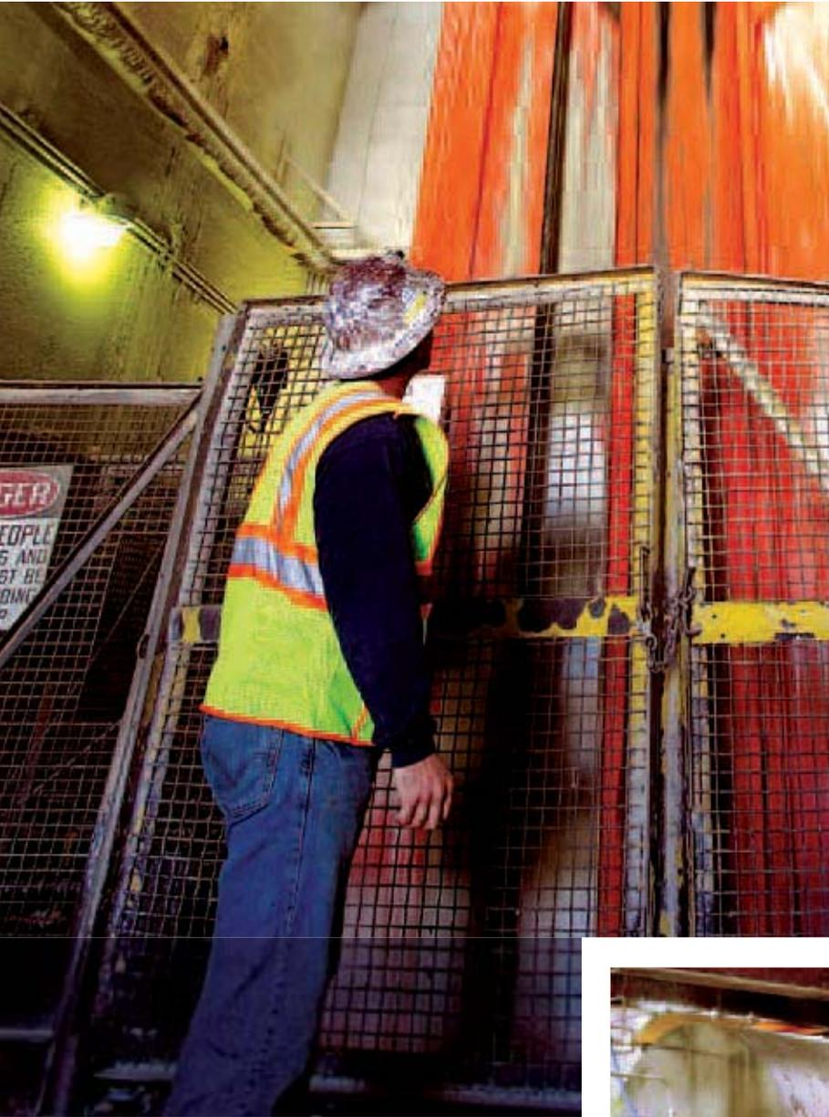
**A** worker oversees the mined trona being transported to the surface, and daylight, by a skip. All the mined ore goes to the surface through such skips, which receive the mineral from the bin — 22 tonnes of it every 90 seconds, 24 hours a day.
