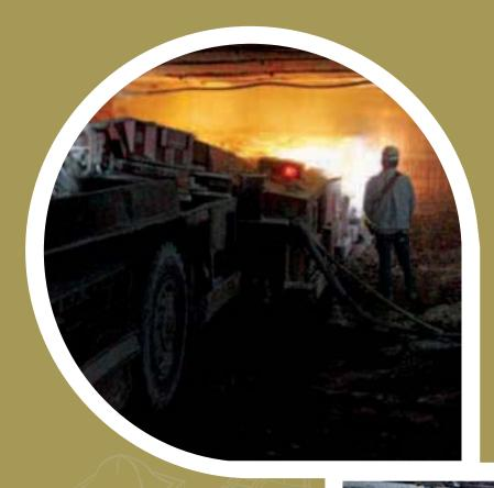
continuous miner, less productive but more flexible than a bore miner, fetches the trona and deposits it in a shuttle car, from where it is transferred to a conveyor belt. The Green River facility sits on the 'mile-high' prairies of southwestern Wyoming, home to the largest reserves of trona ore in the world — 60 billion tonnes spread over 1,000 square miles, at depths of up to 1,800 feet.
