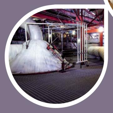
ith shale and other contaminants removed from the liquid substance obtained in the purification process, the water used to dissolve the ore can now be removed. Evaporators, such as those seen here, boil the solution, leaving behind soda ash crystals. These crystals show up as a kind of slurry. Any remaining water is separated from the crystals in a centrifuge
