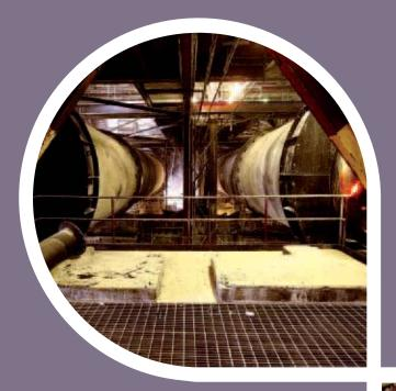
alciners — huge containers in which a substance is heated to a high temperature, but below its melting point — heat the precision-crushed trona to 165°C. This is done to get rid of unwanted gases and some other impurities from the ore; the heating process transforms it into crude sodium carbonate. Each calciner can process about 130 tonnes of trona in an hour.
